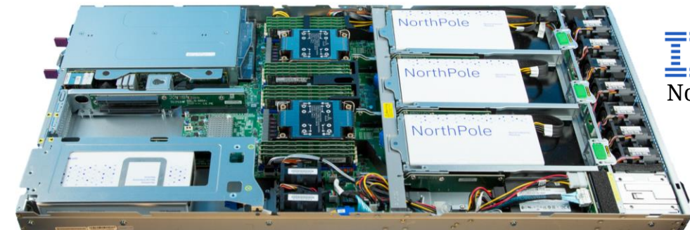
NorthPole scale-out assembly (Prototype)
